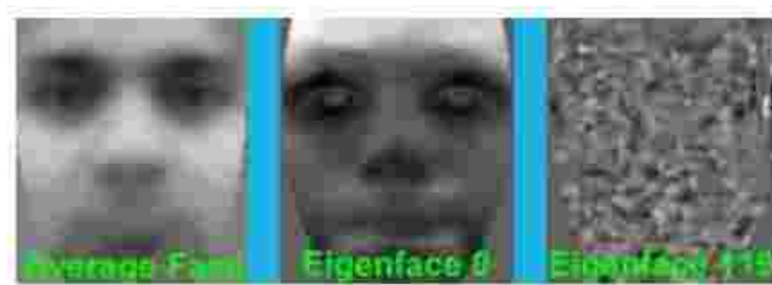
Figure 2. 7 The average face, the first and last eigenface which is mainly noise
